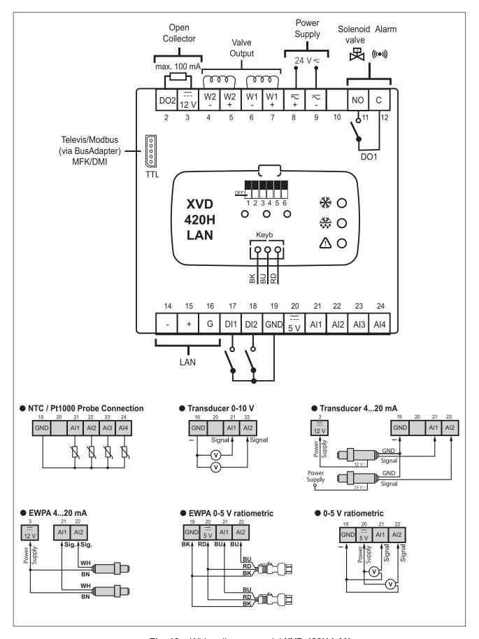
Fig. 12. Wiring diagram model XVD 420H LAN
