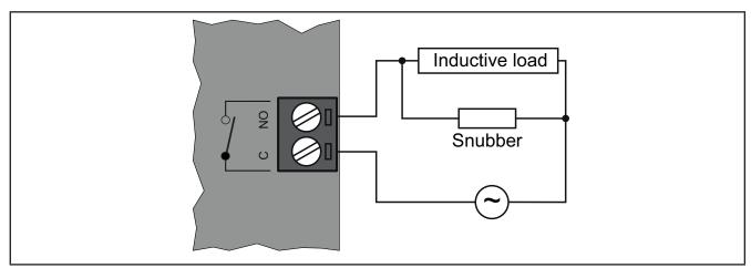
Fig. 10. Protection circuit A
