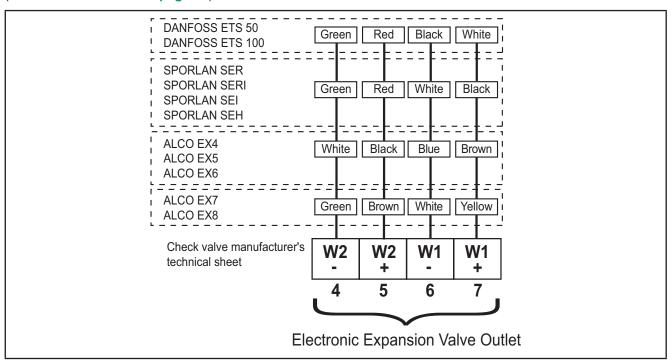
Fig. 18. Connection diagram of pilotable valves
