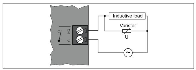
Fig. 11. Protection circuit B
