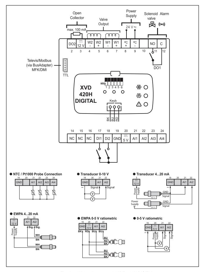
Fig. 14. Wiring diagram model XVD 420H DIGITAL
