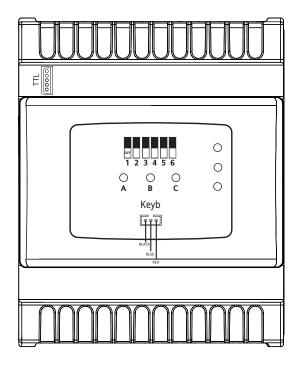
**NOTE**: To connect the MFK to the TTL serial port, use the yellow cable supplied.
