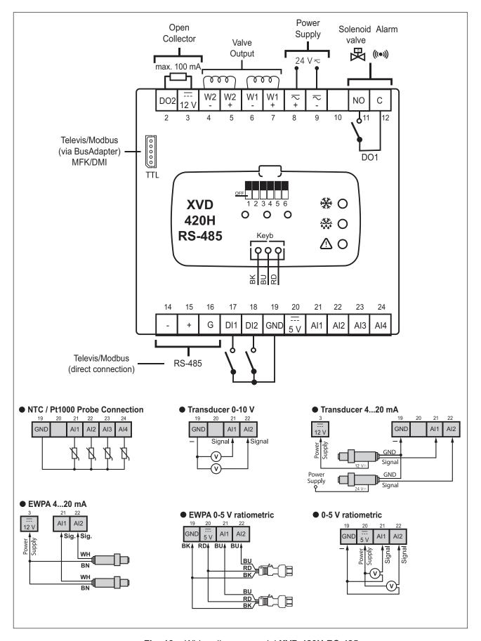
Fig. 13. Wiring diagram model XVD 420H RS-485
