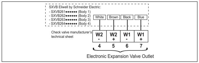
Fig. 17. Connection diagram of compatible valves
