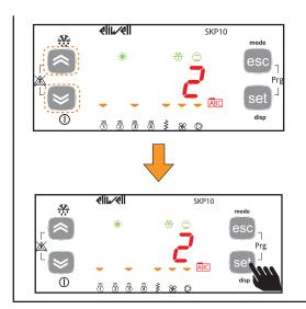
For parameter dL01, the value shown will be 2. To change the parameter value, press the "UP" and "DOWN" keys.
