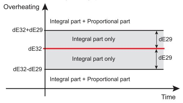
The proportional component is equal to 0% within the thresholds while it cuts in outside of these.
