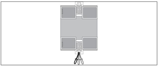
Fig. 2. Detail of sping hooking devices
