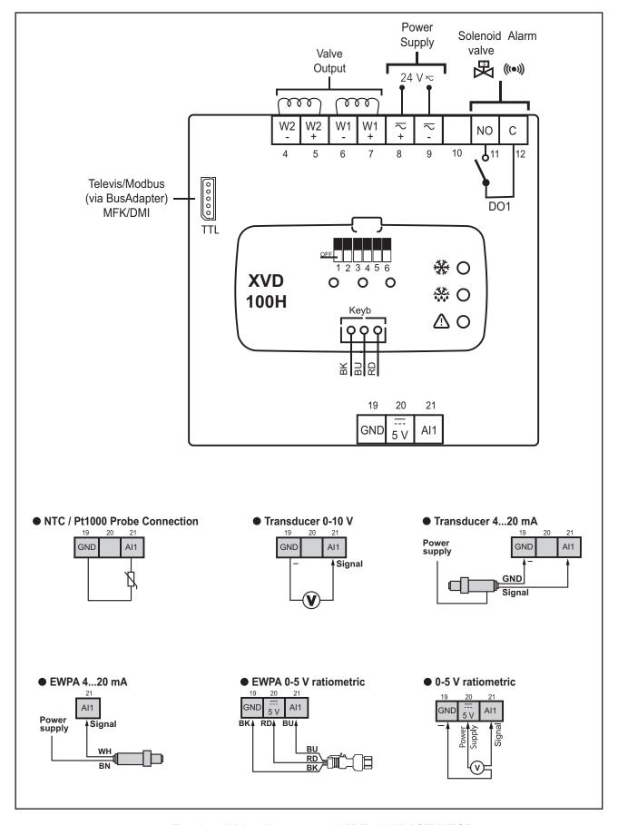
Fig. 15. Wiring diagram model XVD 100H ACTUATOR
