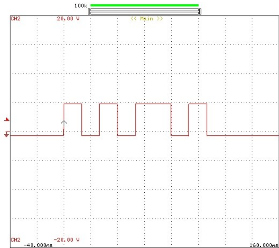
Figure 32 - Signal example of an A5h sent to Inverter.
