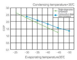
Compared with single-stage compressor, the compound twostage screw compressor is more advantageous in the energy efficiency under low temperature conditions, and reducing the operation cost.
