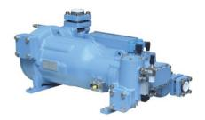
1 x SRMTec C2NA14M-VDMV semi-hermetic duo-compressor-pack with Qo: 575 kW capacity cools the ice hockey arena directly by flooded ammonia circuits.
