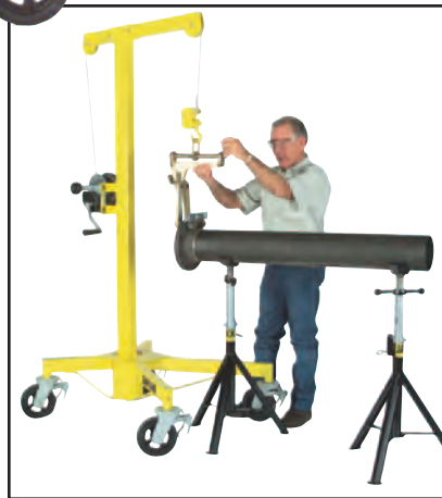
Align flanges with Sumner Adjust-A-Flange
